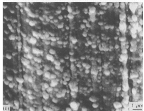
Figure 9 Scanning electron micrographs of (a) the interior area and (b) drawn fibre surface with 1.5 mol% \text{Al}_2\text{O}_3 .
